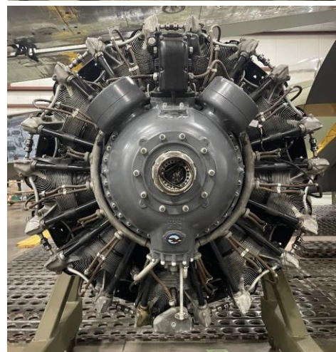
Pratt & Whitney Double Wasp R-2800. On display at the New England Air Museum. Author's Photo.
