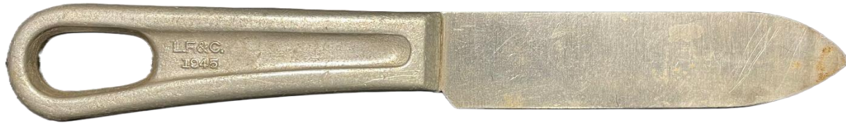
My Grandfather's WW2 mess kit knife made by Landers, Frary & Clark in 1945. Stamped L.F.&C. on the handle. WWI models would have a straight handle without the hole.
